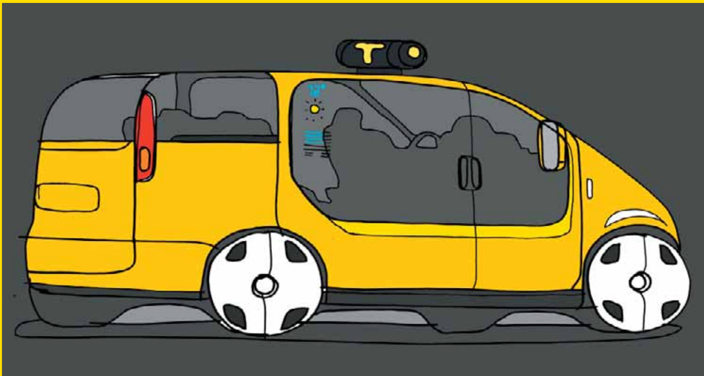
left: BIRSEL + SECK The welcoming doors and high roof on this Birsel + Seck design ease passenger entry.
