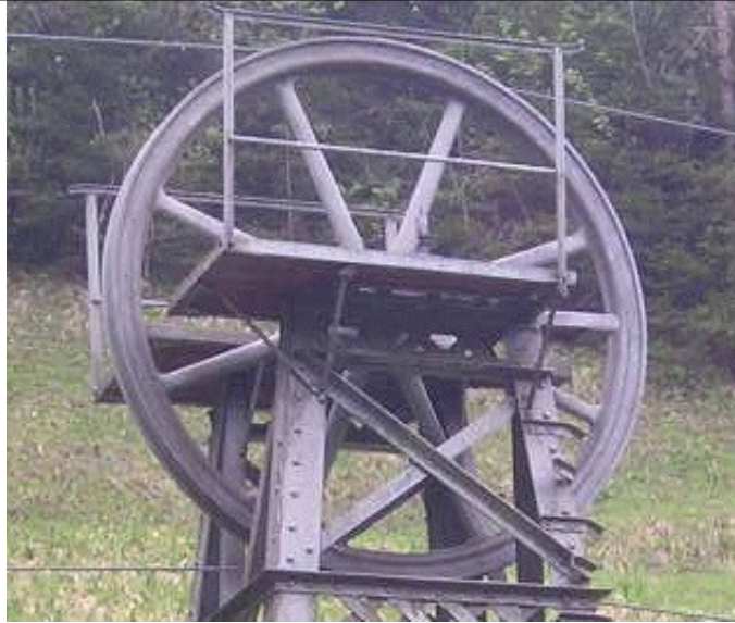
Pulley wheel of the wire rope transmission in Neuthal, Switzerland. Picture credit.
