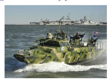
Sailors assigned to Riverine Group 1 conduct maneuvers aboard Riverine Command Boat (Experimental) (RCB-X) at Naval Station Norfolk. The RCB-X is powered by an alternative fuel blend of 50 percent algae-based and 50 percent NATO F-76 fuels to support the secretary of the Navy's efforts to reduce total energy consumption on naval ships. (U.S. Navy photo by Mass Communication Specialist 2nd Class Gregory N. Juday).
