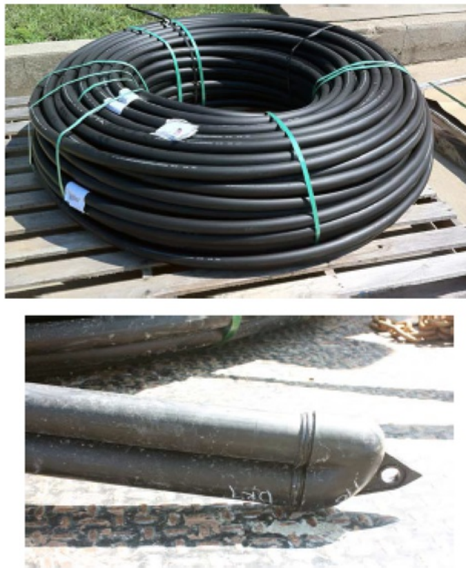
Figure 3. The polyethylene tubing and the metal end fixtures for insertion into the MS&T boreholes. (MST)
