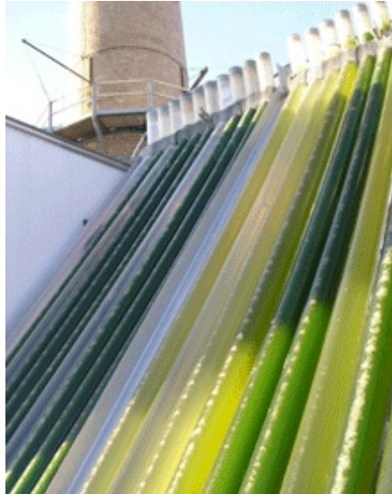
Smokestack emissions bubble through algae-filled tubes at MIT's Cogen plant (from LOE)
