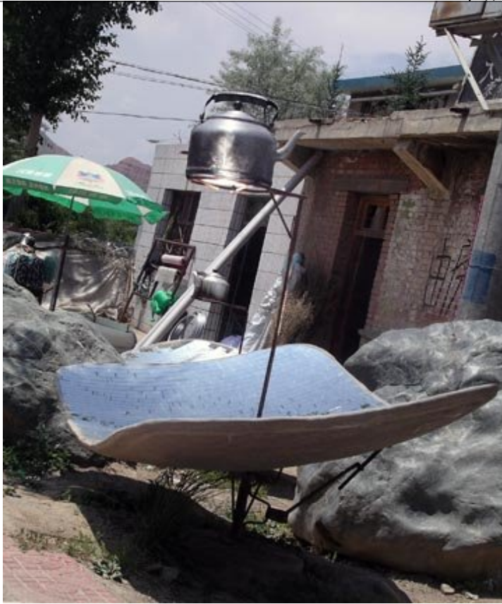
Figure 6. Solar heating of a kettle (30 min to boiling)
