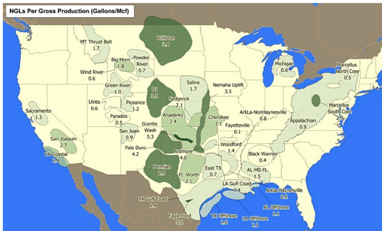
Figure 5. Volume of NGL produced per kcf of natural gas in different fields around the United States ( NPC North American Resource Development Study ) (PDF)
