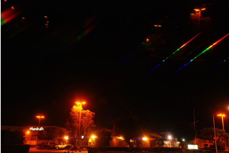
Figure 3: A low-pressure sodium vapor lamp over a tree is almost perfectly monochromatic, as seen by the single, sharp spectral image at upper right. A much weaker green line is also barely visible. Two other LPS sources in the lower-left of the picture are seen in their monochromatic spectral form near the upper-right.
