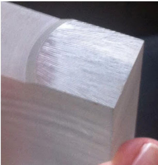
Figure 7. Surface of a crack grown out slowly from the initial notch (finger for scale)
