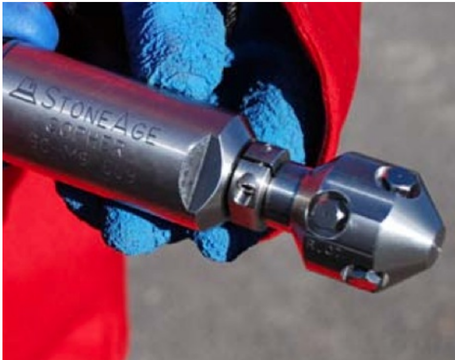
Figure 2. StoneAge "Gopher" showing the nozzle array at the front of the tool ( StoneAgeTools )
