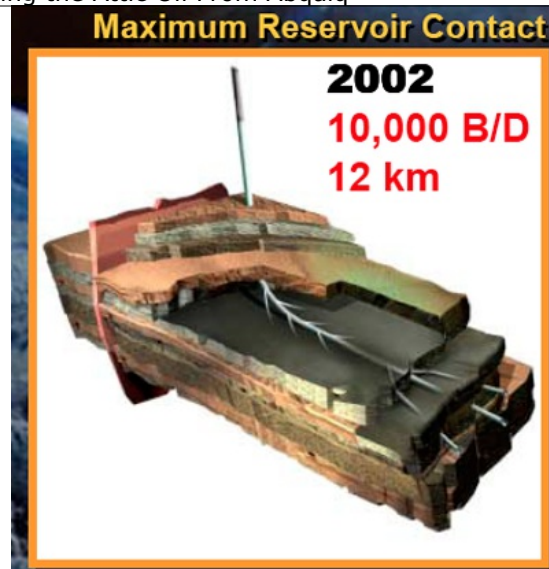
Figure 3. Initial MRC pattern of laterals used at Shaybah (Baqi and Saleri, 2004)
