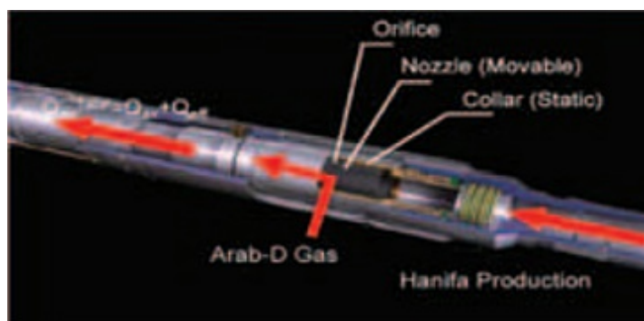
The use of the gas cap to power production from the Hanifa at Abqaiq ( Al-Otaibi et al )
