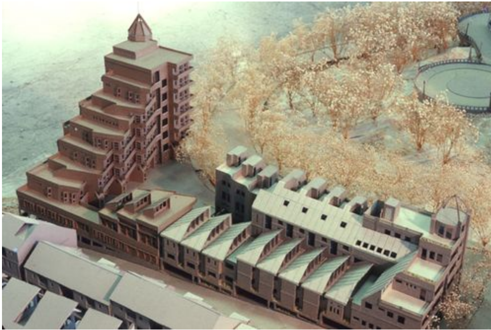
Building designs under the solar envelope are characterised by roof terraces, courtyards and clerestories. Ralph Knowles.
