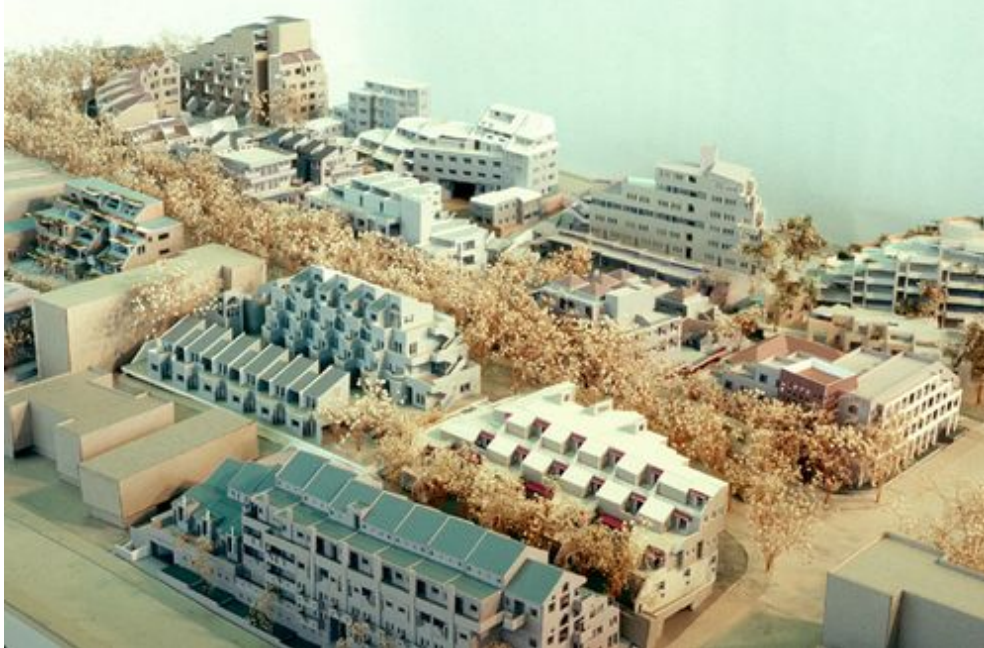
Buildings under the solar envelope on the Spanish grid in LA, reaching densities up to 72 du/ac. Ralph Knowles.
