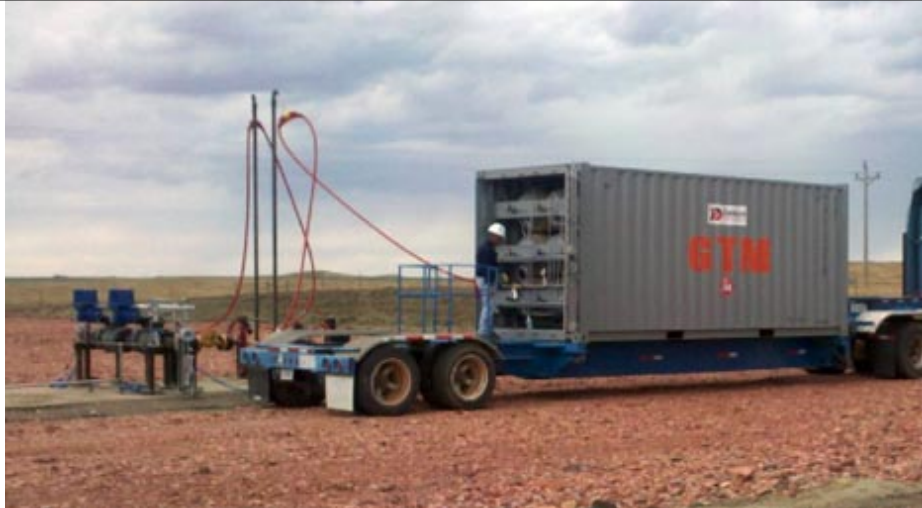
Truck used to transport CNG (Bakken Express)
