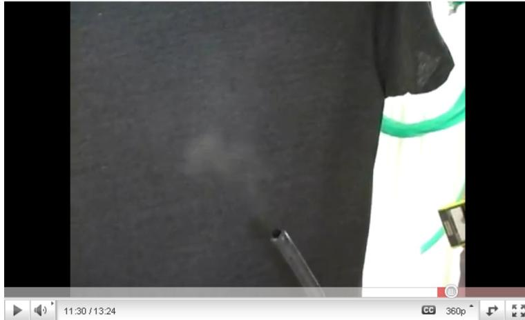
*The "Energy Catalyser" (E-Cat) is a device that has been [reported by two Italian scientists](#) to be able to solve the world's energy problems by means of a nuclear fusion reaction. Unfortunately, there are [serious doubts](#) about these claims. In the figure above (from [a paper by Peter Ekstrom](#)) you see one of the problems with the E-Cat: the trickle of the steam produced by the device in operation is way too small to indicate that it actually produces energy.*
