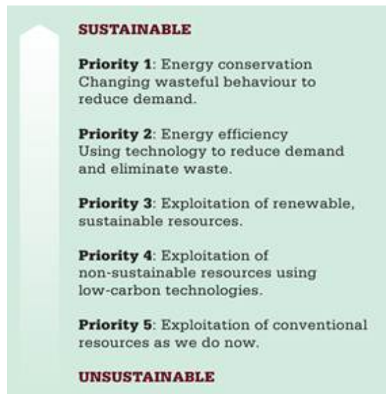
The energy hierarchy, according the Institute of Mechanical Engineers ( ImechE, 2009 )
