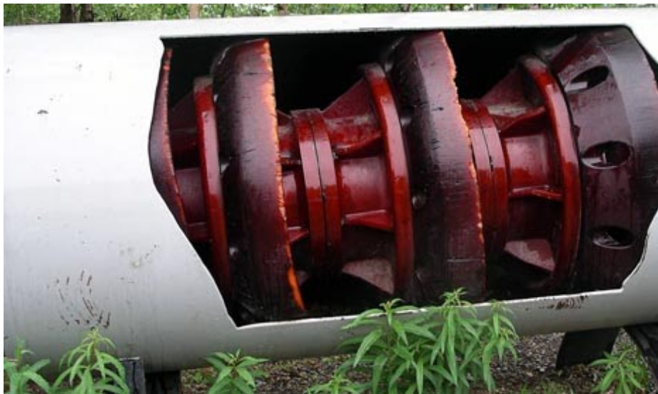
Example pig used in the Alaskan pipeline – see the wipers and note the central compartment within the pig.
