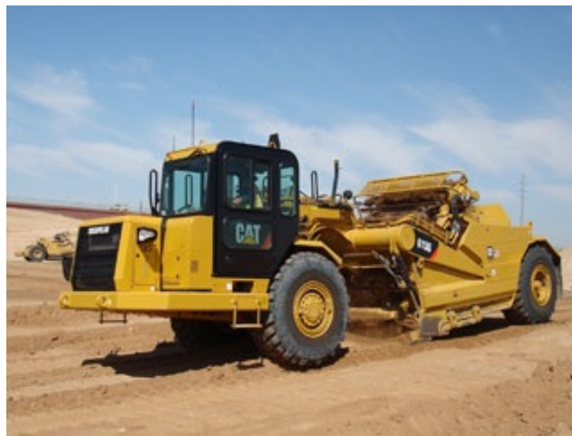
Scraper that could be used to remove and replace soil (Source Caterpillar ).
