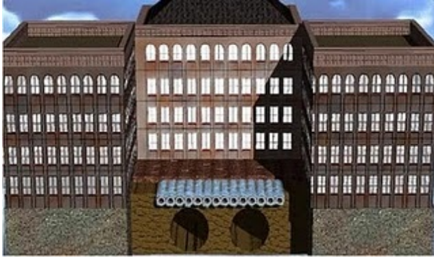
Ice wall as temporary support (image Joe Summers)
