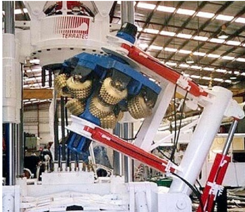
Reaming head being loaded into place.
