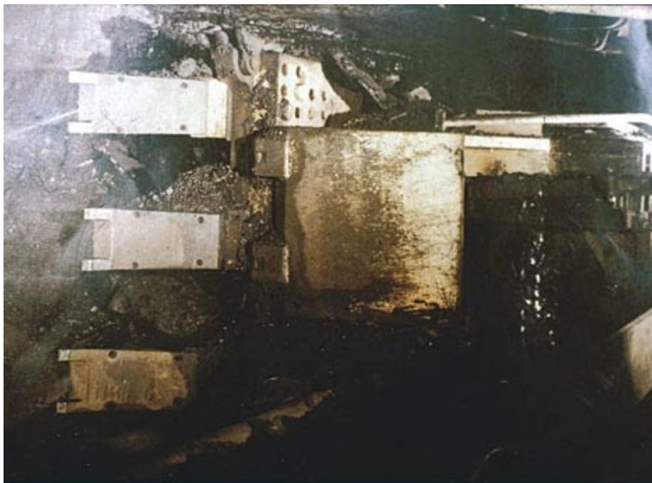
Waterjet plow operating underground in Germany (from Gluckauf)
