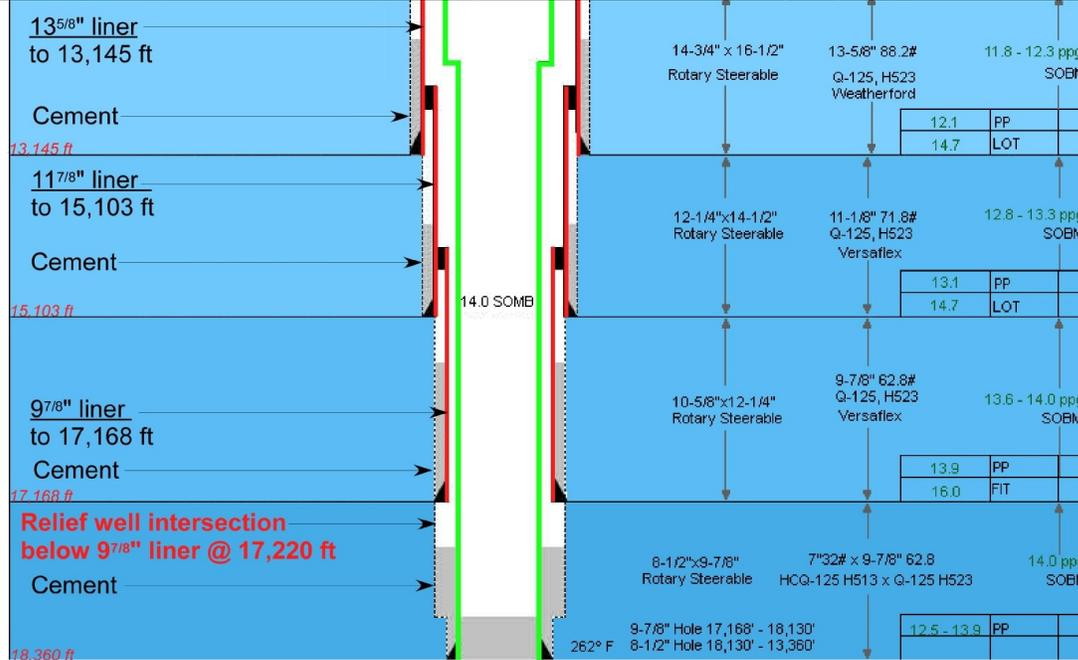
Figure 1b. Lower portion of Department of Energy well configuration diagram. Modified from [http://www.energy.gov/open/documents/3.1\\_Item\\_2\\_Macondo\\_Well\\_07\\_Jun\\_1900.pdf](http://www.energy.gov/open/documents/3.1_Item_2_Macondo_Well_07_Jun_1900.pdf)
