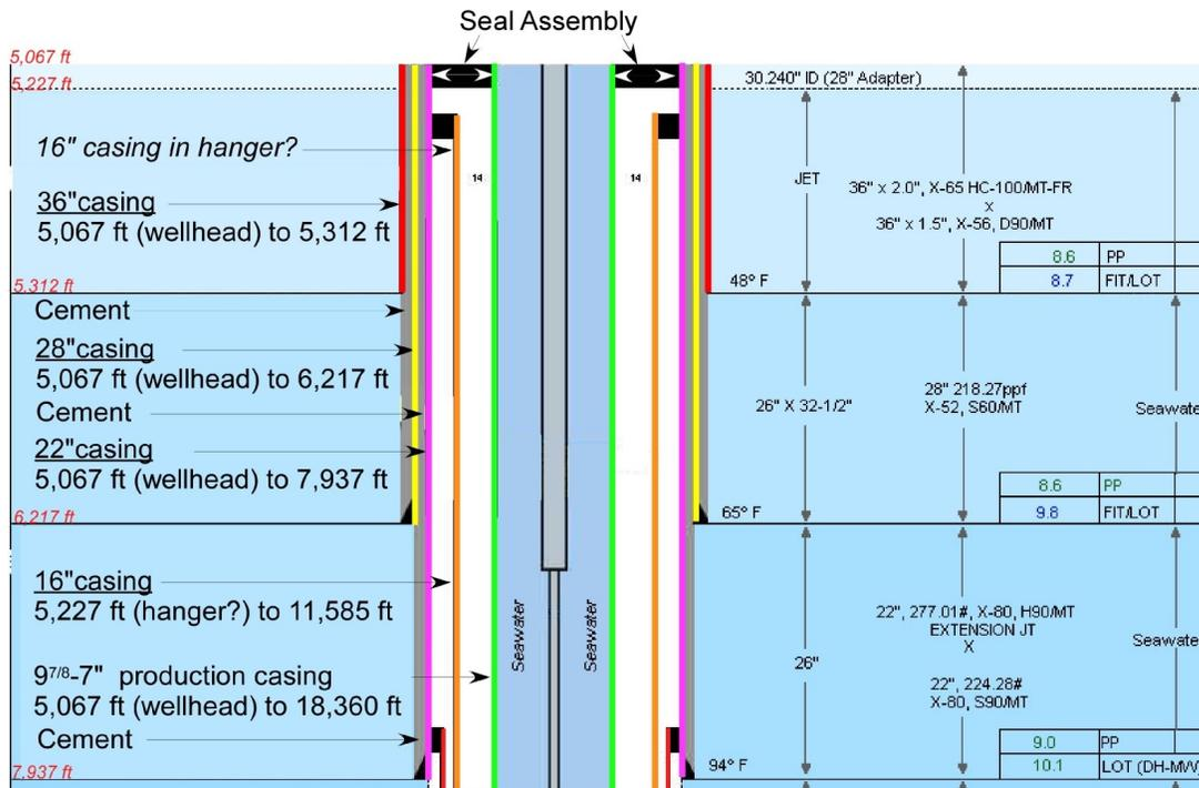
Figure 1a. Upper portion of Department of Energy well configuration diagram. Modified from [http://www.energy.gov/open/documents/3.1\\_Item\\_2\\_Macondo\\_Well\\_07\\_Jun\\_1900.pdf](http://www.energy.gov/open/documents/3.1_Item_2_Macondo_Well_07_Jun_1900.pdf)
