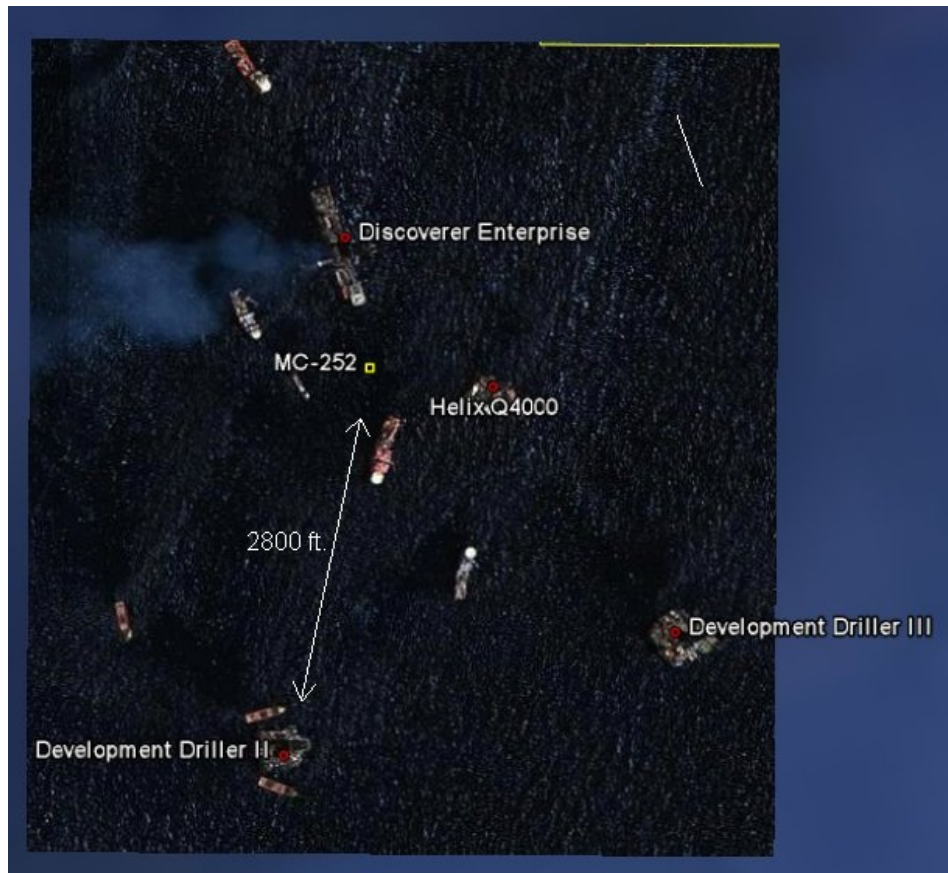
Figure 1. Satellite photograph (DigitalGlobe) showing relief well rigs and oil containment ships operating on May 24, 2010. Location of MC-252 well on photo ascertained using coordinates from DigitalGlobe measurements and the Macondo well plan and drilling authorization submitted to MMS by BP.
