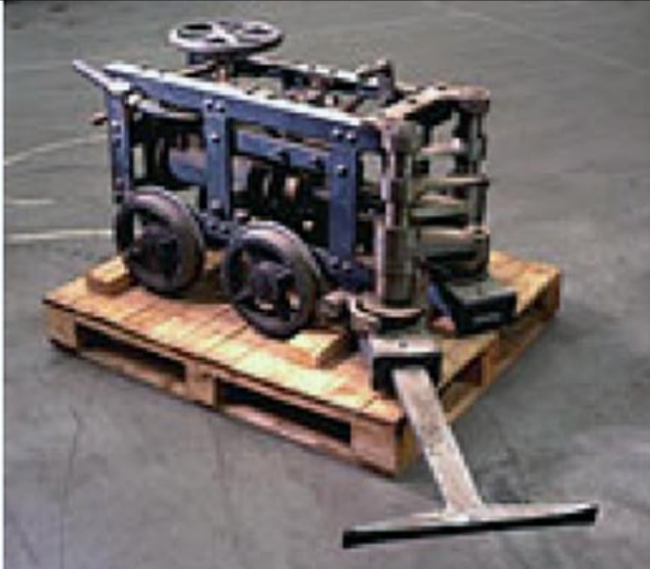
Early coal cutting machine used at Garth Colliery in Wales in 1863. ( National Museum Wales )
