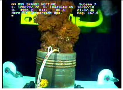
Flow from the top of the 3-ram stack at 10:45 pm Eastern Monday – the color is due to the injection (through the white feed) of the dispersant into the flow.
