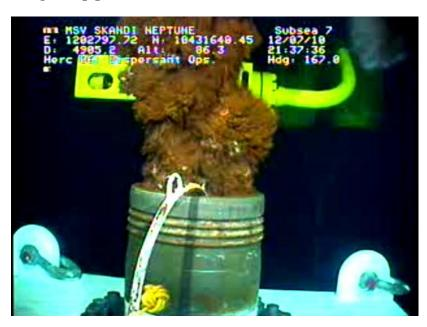
Flow from the top of the 3-ram stack at 10:45 pm Eastern Monday – the color is due to the injection (through the white feed) of the dispersant into the flow.
