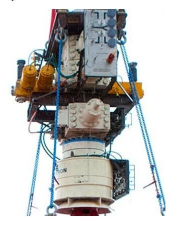
And this is the main control panel, with the ability to operate the valves with the ROVs made rather evident. I suspect this picture was taken a little while ago, and the port cut for a valve with a cutting torch has been cleaned up a little since then.
