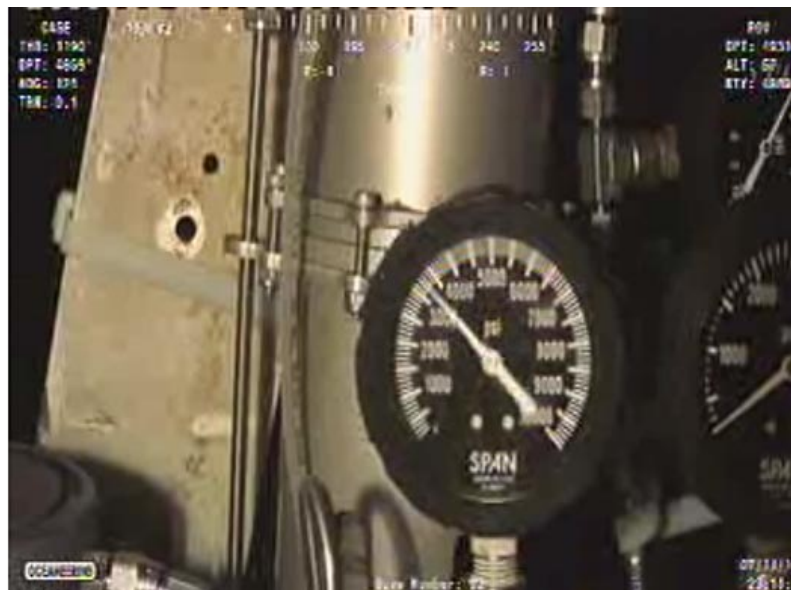
Pressure gage (which goes up to a pressure of 6,500 to 7,000 psi)
