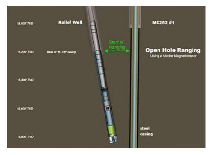
The instrument package is then run into the hole with a Vector Magnetometer, which is mounted on a wire to carry it in and out (known as a wireline). The process of drill and test, using the Magnetometer, continued until the steel casing in the original hole had been detected.
