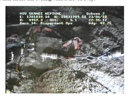
Skandi ROV1 showing the electrical connections (lhs) to the plate allowing the electrical pulses to be transmitted down the casing.
