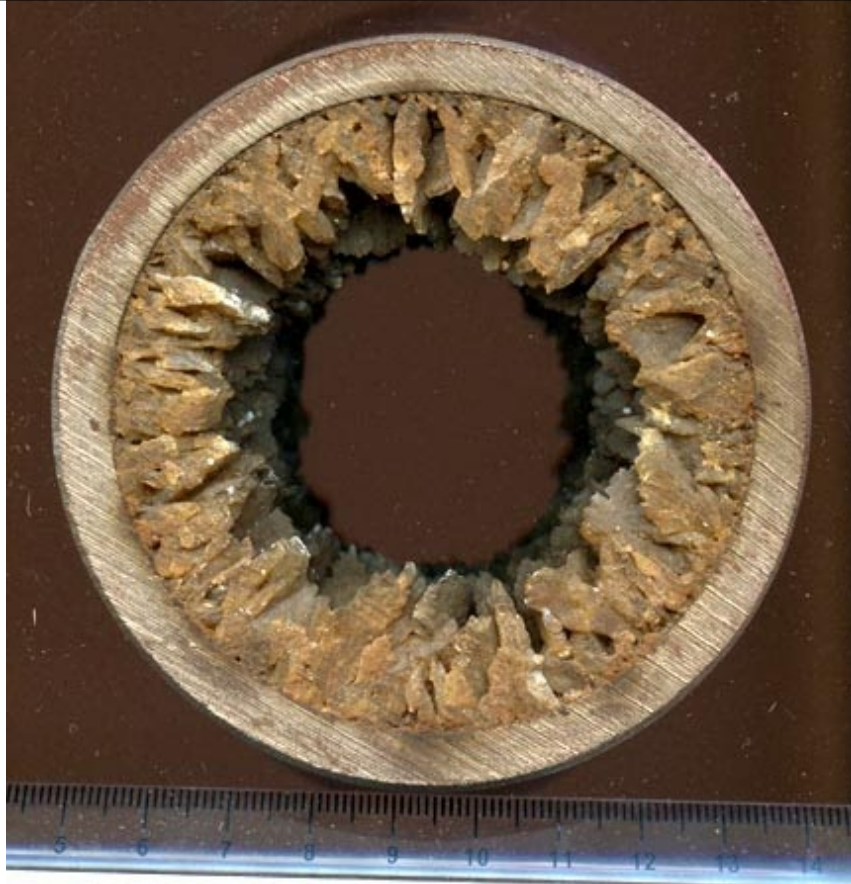
Barium Sulfate Crystals growing in a 3-inch I.D. pipe that carried oil from the deposits under the North Sea. (Scale is in cm) (Growths of this size can occur in less than 24 hours).
