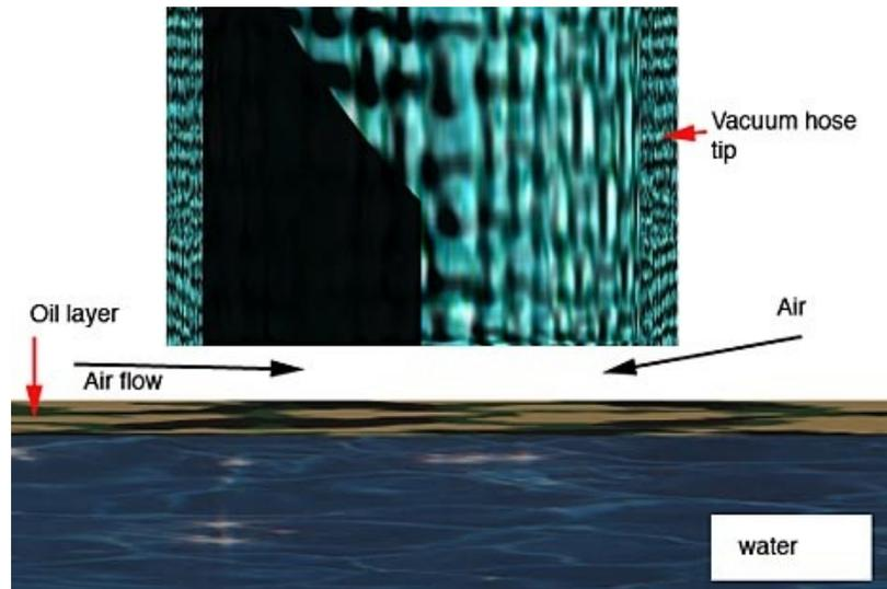
Unless you have really good control of your position (bearing in mind you are looking along the hose at the water) this is very hard to sense. If you push the hose into the water hardly at all then you pull in too much water and not that much oil.
