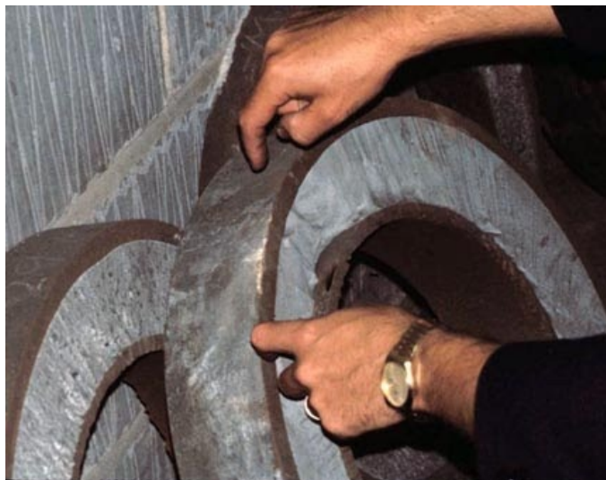
ASJ cuts of casing from the bottom of the North Sea
