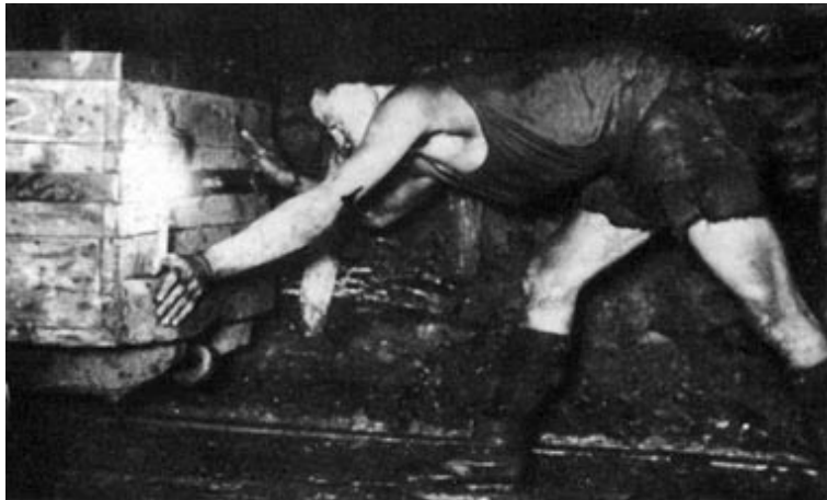
Putting in a 2 ft 10 inch coal seam, 1929 (A Bevin Boy Remembers, Ted Holloway, Henge Publications, 1993)
