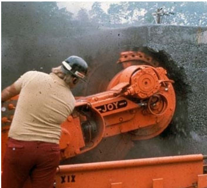
Surface test of a shearer used in longwall (Bureau of Mines Bruceton)
