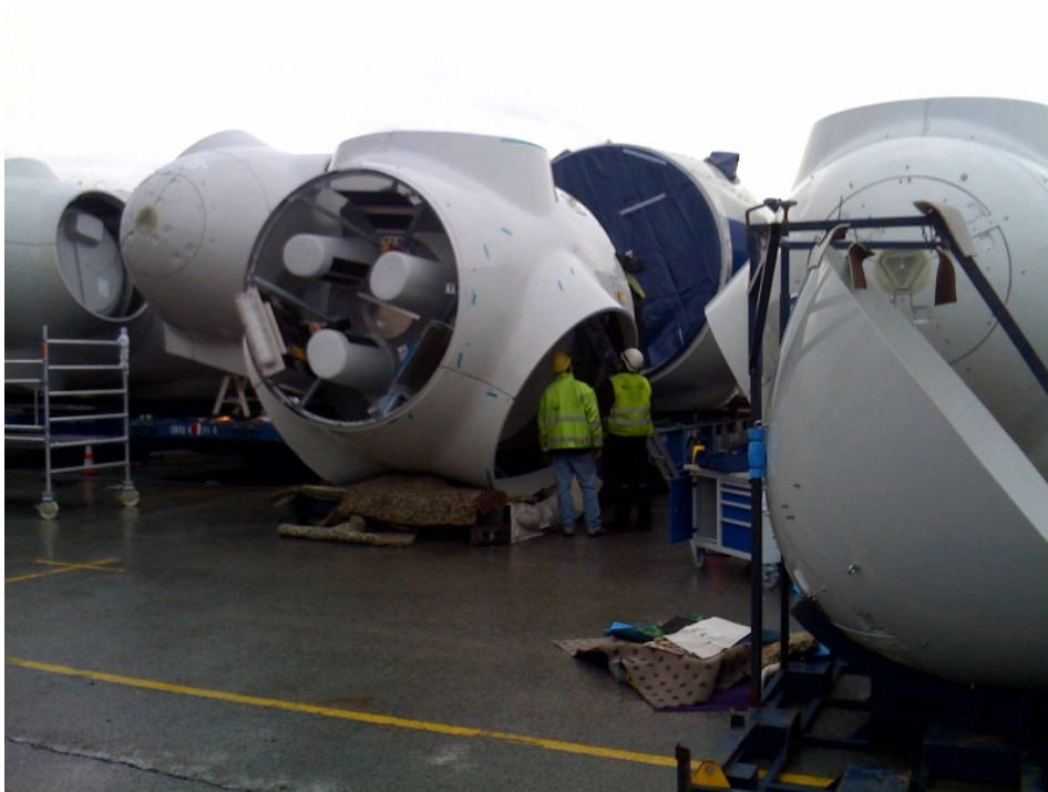
The hubs are first positioned alongside the nacelles
