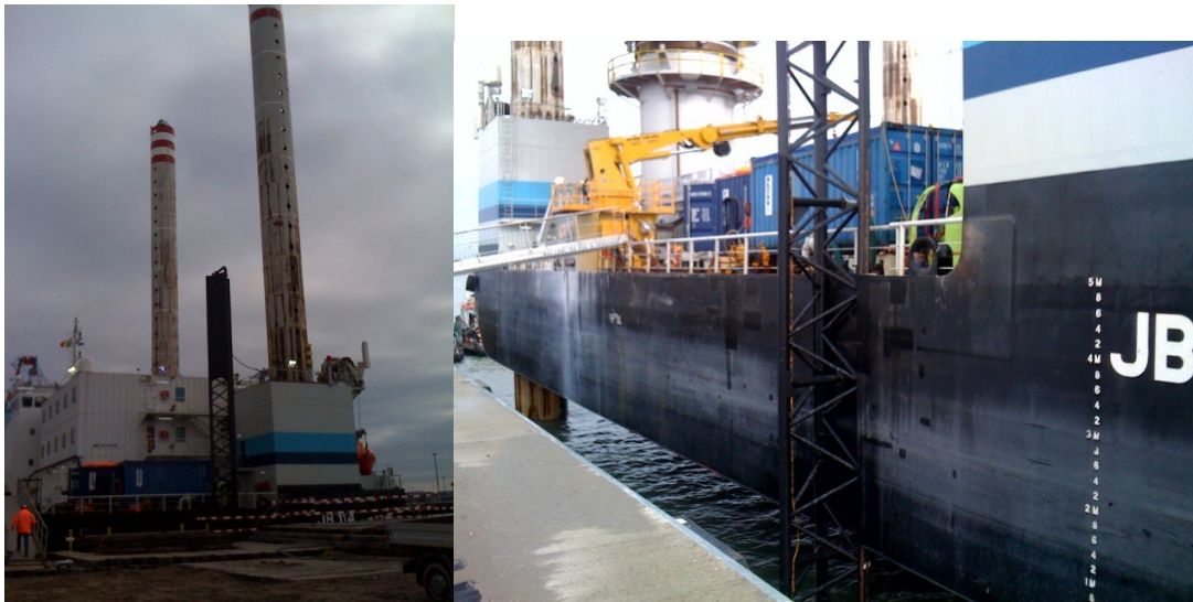
Left: two of the legs that go down in water to lift the platform above the water when it needs to work
