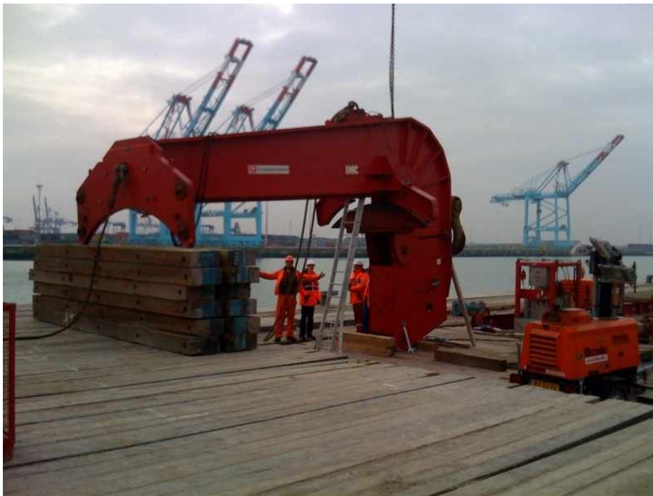
this is the special piece of equipment used to "grab" foundations and bring them from their horizontal transport position to the vertical on site. It was temporarily on site for some repairs/maintenance.
