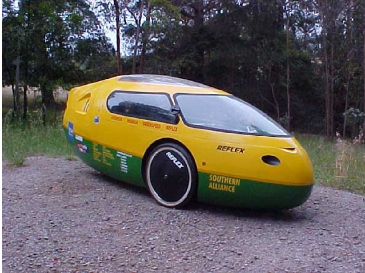
Figure 5: Velomobile fairings can reduce a typical cyclist's C_d from 0.9 to 0.012
