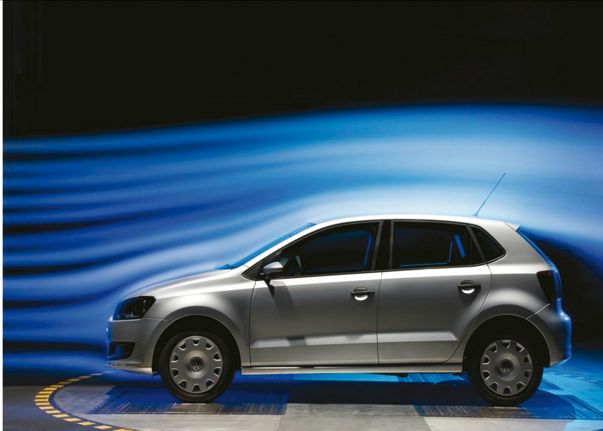
Figure 4: Wind Tunnel testing of the new VW Polo
