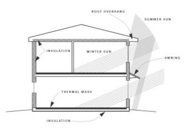
Direct Gain heat transfer (Graphic courtesy of RecycleWorks)
