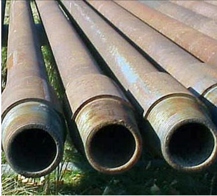
Normal male pipe ends (taped over to protect the threads)
