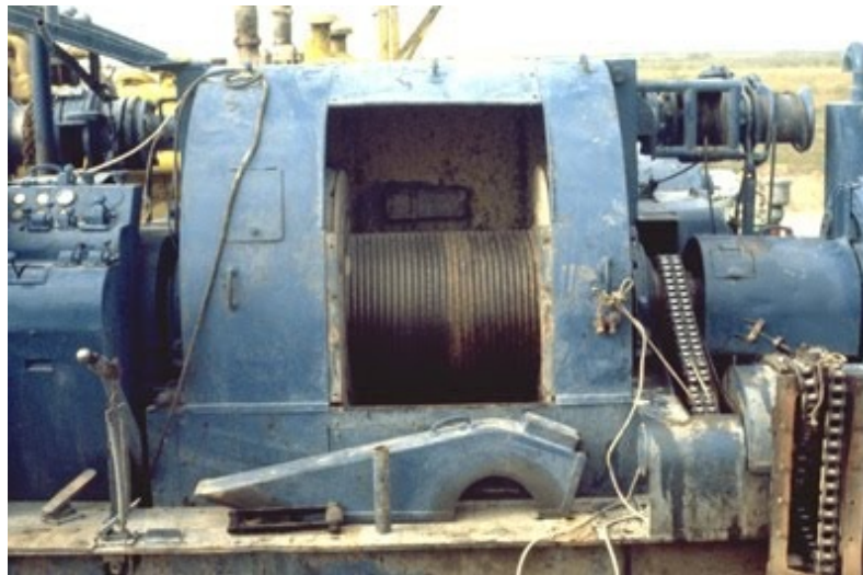
The hoist and motor of the Drawworks ( Schlumberger )
