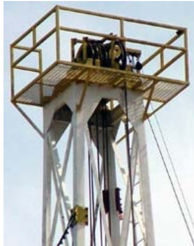
Crown block at top of mast ( OSHA )
