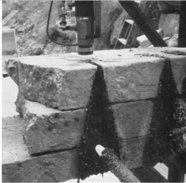
Cut into rock using a plasma to melt the rock ( US Bureau of Mines )
