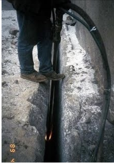
Hand-held flame jet cutting a slot in granite. Note the slot width and the flame at the bottom of the lance. (These can cut about 14 sq. ft/hour of slot)
