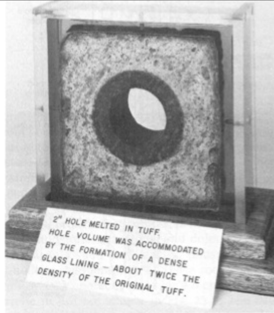
Resulting hole drilled by the Subterrene.
