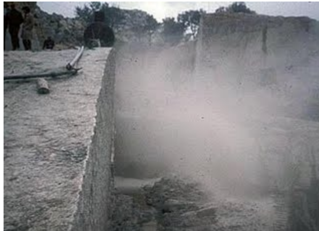
Cloud of fine particles created when a jet burner cuts a slot into a granite block.
