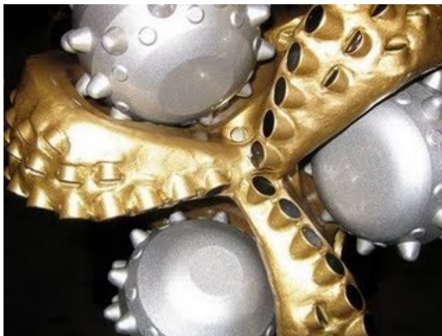
Large drill bit combining the buttons of a tri-cone (the silvery points) with polycrystalline diamond cutters (the dark circles). ( Source )
