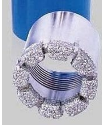
Diamond coring bit, the dark specks are individual diamonds ( Source )
