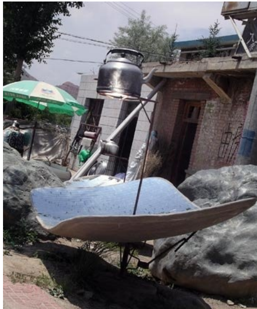
Solar heating of a kettle (30 min to boiling)
