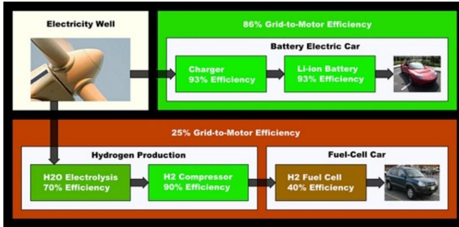
The diagram above shows that both the efficiency of electrolysis and the efficiency of fuel cells are key factors in making hydrogen as a transport fuel less attractive than the electric transport option.
