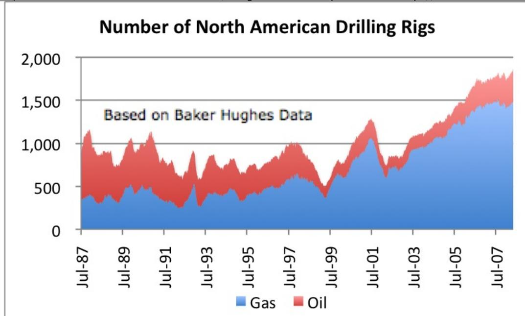
Figure 7. Number of North American leased rotary drilling rigs
