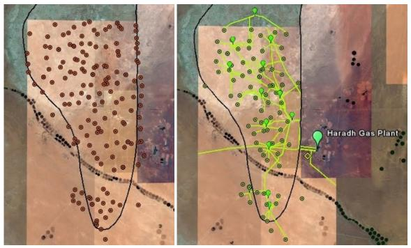
All visible lower Haradh wells (left) and identified gas wells, pipelines, and manifolds (right).
