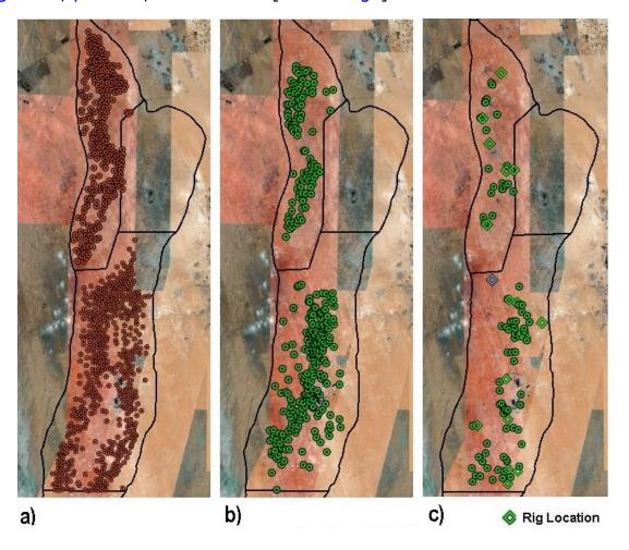
Oil Wells in 'Ain Dar and Uthmaniyah: a) before ca. 2000, b) between 2000 and 2003, and c) developed after 2003 including sites prepared for drilling and those undergoing active drilling in summer 2006. Water injectors are not shown. Source: Satellite O'er the Desert.
