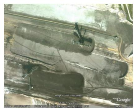
The coal mine of Garzweiler, Germany, in a Google Earth image. The satellite has caught two giant mining machines at work. Measured with the google ruler, each "arm" of the machines measures about 120 m (ca. 400 ft). These are not universal mining machines, but give some idea of the scale of modern mining operations. The Garzweiler mine is said to hold more than a billion tons of coal reserves.
