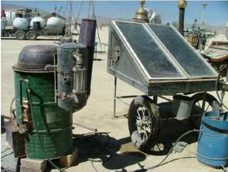
Another fun solar application was "Dr. Blendo's Solar Powered Smoothie Machine": a DIY project built on a little cart, with an electric and a hand-powered blender, a canopy of thin-film solar, a Xantrex "Power 1500" integrated battery/inverter unit in the bottom, a Bose sound system, and a cooler. According to Dr. Blendo, the blender overheated and gave out long before the solar power system did. He was using it to charge up all matter of batteries since it was generating extra power.
