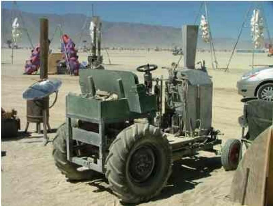
The box in the back contains wood, which is fed into a small firebox at the driver's feet.
