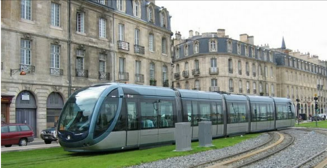
High-tech, style, low-floor comfort in one: a Bordeaux tram (an Alstom type Citadis302) on a catenary-free section at Quai Richelieu, August 16th, 2004. Photo by P.Chapar from RailFanEurope.net
