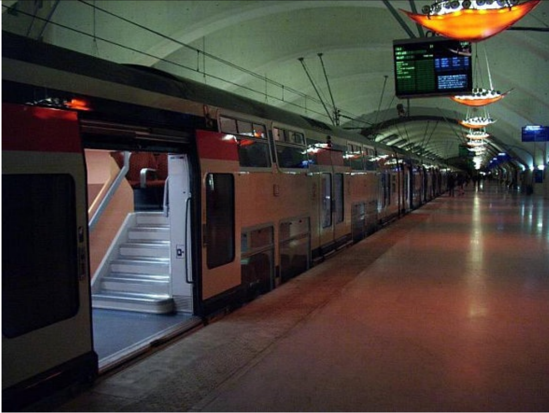
Extreme capacity: lots of wide doors and two levels of an SNCF MI2N (series Z 22500) EMU at Hausmann-St-Lazare station, on the underground part of line E, January 1st, 2000. On line A, two five-car units form a train. Photo by Jörg Kuntz from RailFanEurope.net
