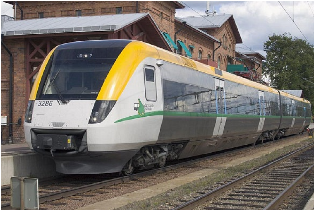
Värmlandstrafik's X53-2 No. 3286, a wide-body electric multiple unit from Bombardier's Regina family, stops as local service in Arvika, May 2004. Photo by Jan Lindahl from SJK
