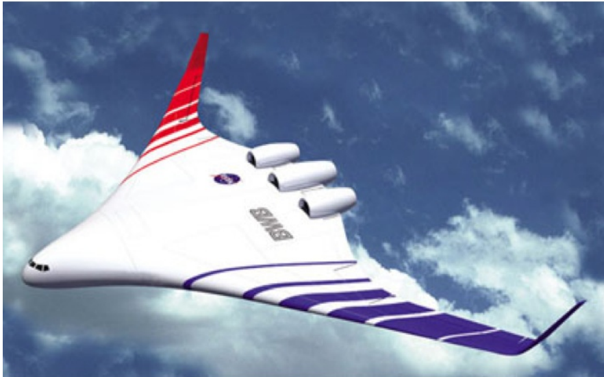
Figure 3. This NASA Blended Wing Body airliner would give a 30% improvement in fuel efficiency over conventional tube and wing designs regardless of the fuel used. Photo: www.nasa.gov/centers/langley/images/content/70059main_2003-81-01.jpg
