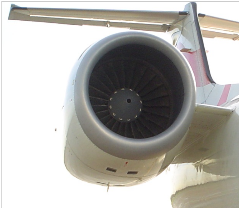
Figure 1. The Allison AE3007A Turbofan (Jet) Engine.
