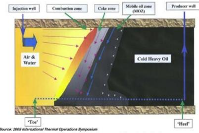
A more advanced technology to recover bitumen in situ, Toe to Heal Air Injection (THAI), is advancing toward commercialization
